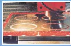
A unique method of vacuum workholding. Ideal for flat, thin and profiled workpieces the patented form of th mat keeps the part securely held down.
